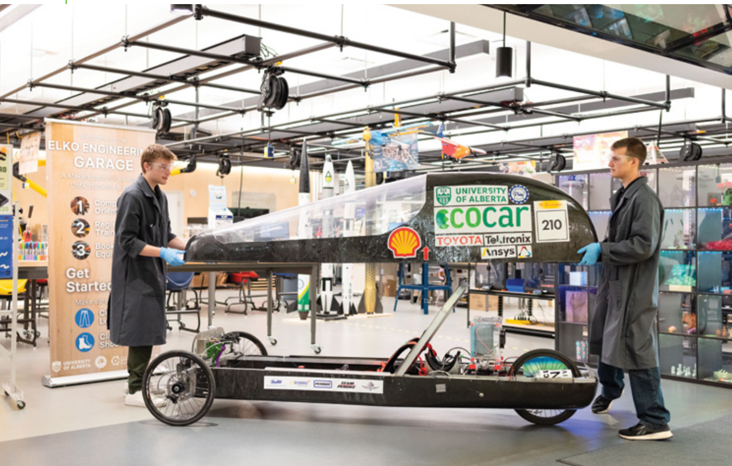
U of A students working on a car powered by a hydrogen fuel cell they have designed and built from scratch.
