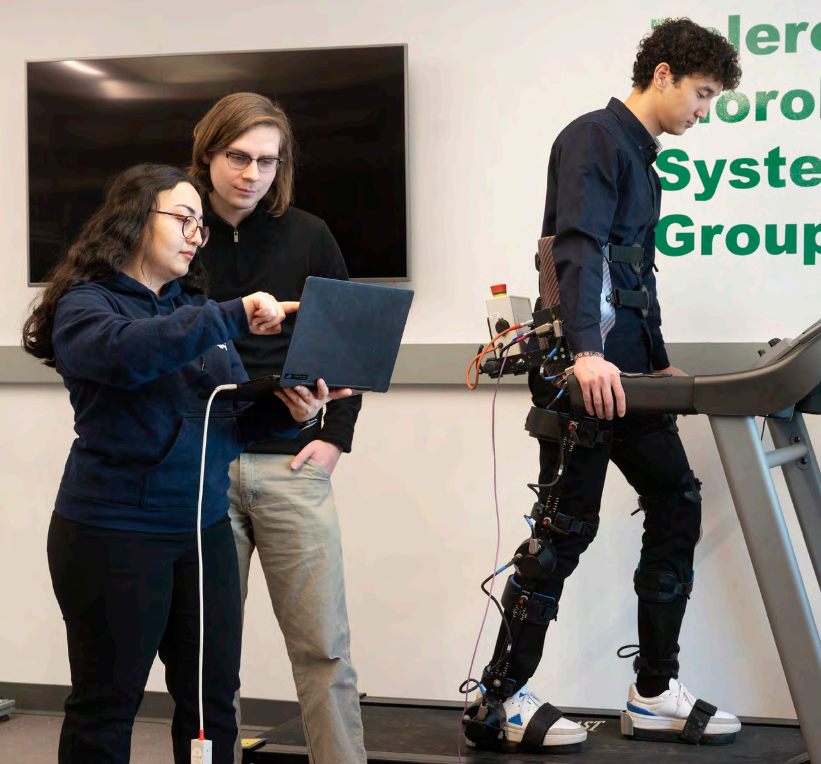
Tleukhan Mussin, walking on a treadmill wearing the lower limb exoskeleton. Maryam Shakourisalim and Andor Siegers monitor progress of the lower limb exoskeleton during walking.
