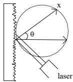
*Example:* Calculate the nominal ocular hazard zone for a diffuse reflection of the ruby laser given in the previous example assuming that the angle of the observer ( $\theta$ ) is 45 deg and the spectral reflectance ( $\rho$ ) is 0.2.
